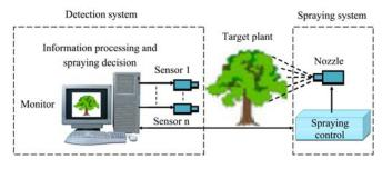
Figure 2 Smart spraying system based on sensing technology
