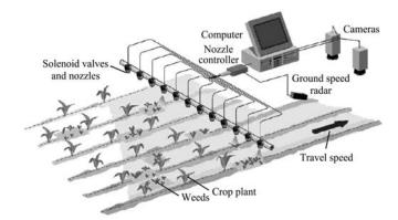
Figure 4 Sprayer system based on machine vision
