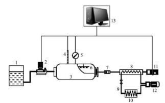
Note: 1. Water tank 2. Water pump 3. Vacuum chamber 4. Thermometer 5. Piezometer 6. Water sprayer 7. Check valve 8. Steam condenser 9. Throttle valve 10. Condenser 11. Vacuum pump 12. Compressor 13. Computer Figure 1 Schematic diagram of the self-developed vacuum cooler
