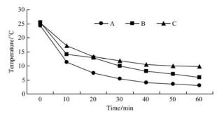
Figure 2 The temperature profiles of broccoli as a function of treatment time according to the vacuum cooling (A), cooling water (B), and cold room (C) treatments
