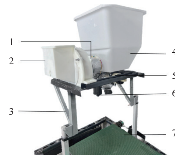
1. Seed dispensing motor 2. Electric drive peanut seed metering device 3. Platform lifting device 4. Fertilizer box 5. Electric-driven peanut fertilizer applicator 6. Fertilizer motor 7. Conveyor belt
