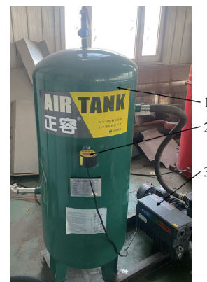
Note: 1. Buffer tank 2. Pressure gauge 3. Vacuum pump
