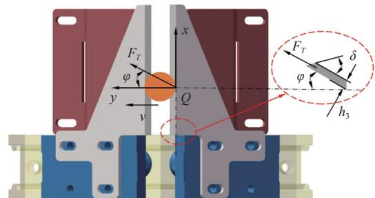
Note:  $\delta$  is inclination angle of the blade, ( $^\circ$ );  $h_3$  is thickness of the blade, mm.
