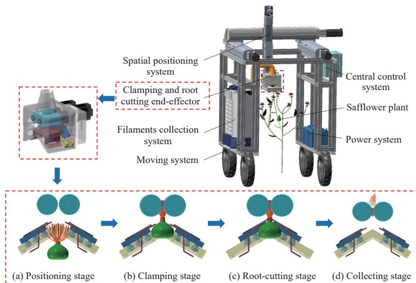
Figure 2 Structure of the safflower harvesting robot
