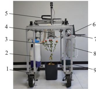
1. Moving system 2. Filament collection system 3. Safflower plant 4. Clamping and root-cutting end-effector 5. Spatial positioning system 6. Computer 7. Vision camera 8. Central control system 9. Power system
