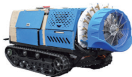
Figure 2 Lanjiang unmanned plant protection robot
