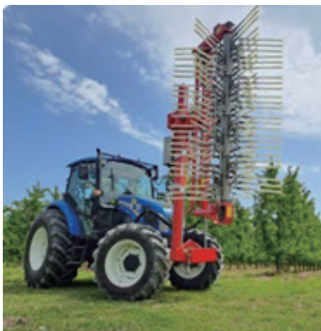
Figure 3 Assirelli vehicle-mounted flexible flower thinning
