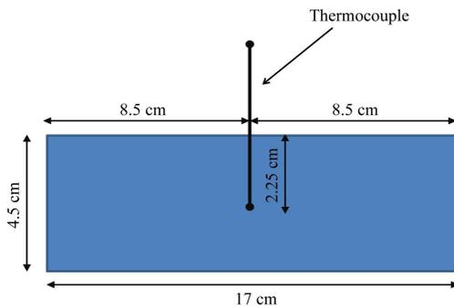
Figure 2 Thermocouple positioning
