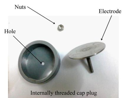
Figure 1 Electrodes of ohmic heater
