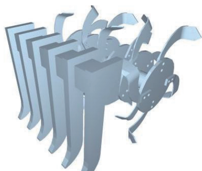
a. Geometric model of soil-loosening mechanism
