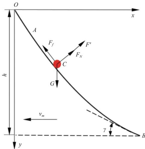
Note:  $F_f$  is the sliding friction force, N;  $F_N$  is the support of the curve to the seed, N;  $G$  is the seed gravity, N;  $F'$  is the seed centripetal force, N;  $h$  is the vertical height of the seed falling, mm;  $\gamma$  is the inclination angle of seed tube end, ( $^\circ$ ).
