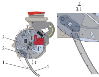
Note: 1.Seed; 2.Seed scraping part; 3.Seed metering plate; 4.Seed delivery tube; I Seed filling area; II Seed clearing area; III Seed carrying area; IV Seed feeding area.
