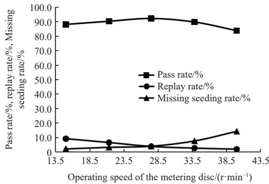
Figure 7 Relation curve between test index and operating speed
