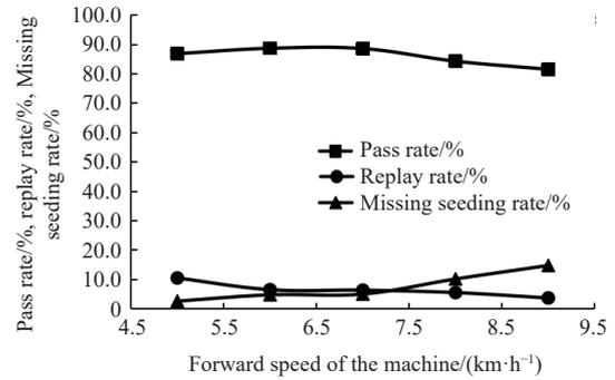
Figure 6 Relation curve between test index and machine forward speed
