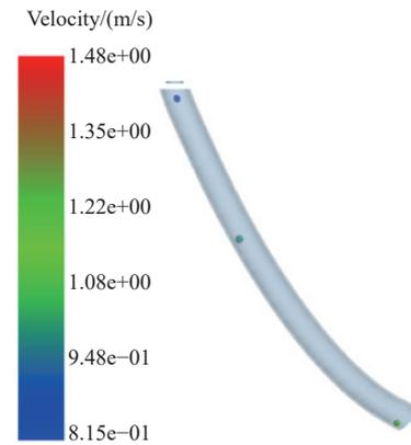
Figure 3 Simulation model of carrot seed guide
