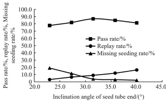
Figure 5 Relation curve between test index and inclination angle of seed tube end
