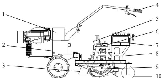
1. Accumulator battery 2. Walking tractor 3. Flat soil slab 4. Pushrod 5. Lifting mechanism 6. DC fan 7. Automatic seed supply mechanism 8. Rack 9. Pinhole wheel type single grain precision seeding device 10. Suppression of wheel
