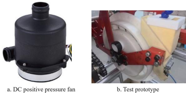
Figure 5 Seed clearing test bench
