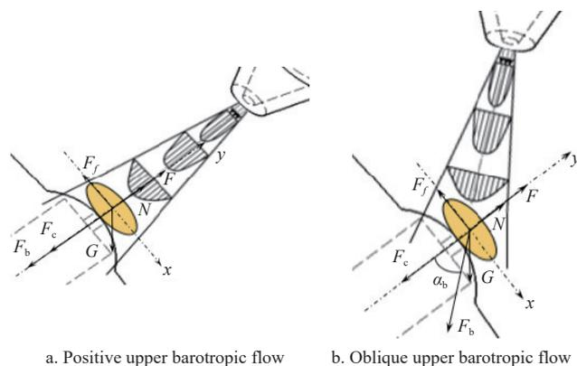
Note:  $F_f$  is the friction force of the pinhole wheel on seeds,  $N$ ;  $N$  is the supporting force of the pinhole wheel on seeds,  $N$ ;  $F$  is the centrifugal force on the seed,  $N$ ;  $F_c$  is the absorption force of seed suction hole on seeds to maintain the seeds being absorbed,  $N$ ;  $G$  is the gravity of seed,  $N$ ;  $\alpha_b$  is the angle of the line of airflow of seed clearing to the suction hole, ( $^\circ$ ).
