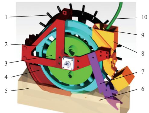
1. Earth wheel 2. Pinhole wheel 3. Force distribution cover 4. Trenching mechanism 5. Soil 6. Seed 7. The soil covering mechanism 8. Seed box 9. Seed suction hole 10. Seed cleaning mechanism
