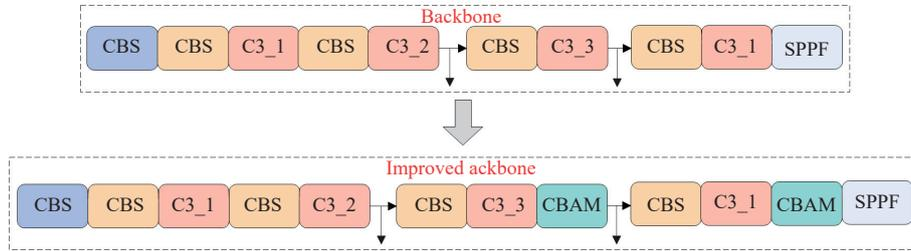
Figure 7 Schematic of the improved backbone network
