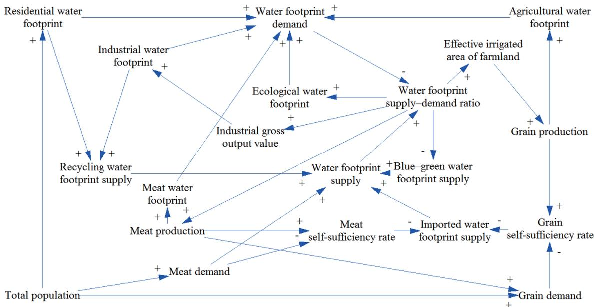
Figure 1 Causal feedback loop diagram of China's water-grain-meat system
