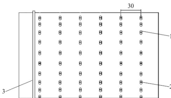
1. Oblong shape cut 2. Around shape (hole diameter 2 mm) 3. Bearing barrier
