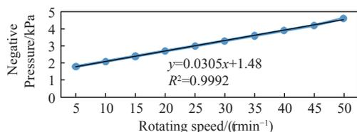
Figure 8 Relationship between rotating speed and corresponding negative pressure for seed pick-up under the six rows
