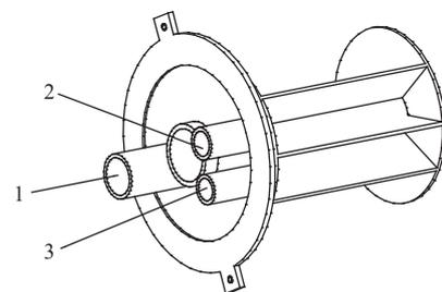
1. Negative pressure inlet 2. Positive pressure inlet 3. Clean out pressure inlet
