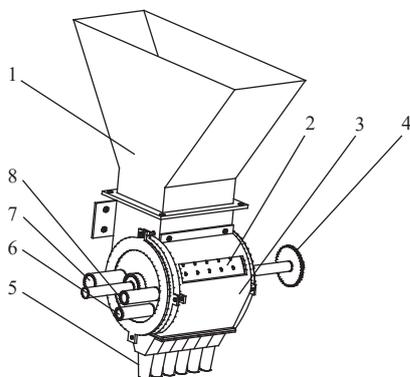
1. Seedbox; 2. Metering cylinder; 3. Removable cover; 4. Driving sprocket; 5. Seed tubes; 6. Positive pressure inlet; 7. Negative pressure inlet; 8. cleanout pressure inlet.
