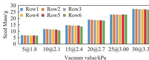
Figure 9 Effect of combined rotating speed and corresponding vacuum on seed pick up under the six rows
