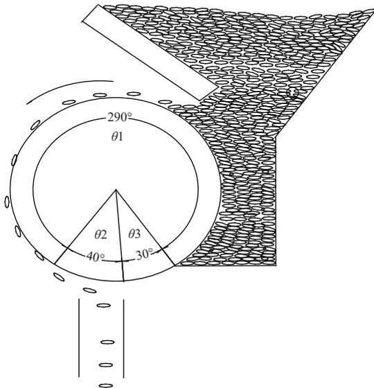
Note:  $\theta_1$ : Picking and retaining angle;  $\theta_2$ : Dropping angle;  $\theta_3$ : Clearing angle
