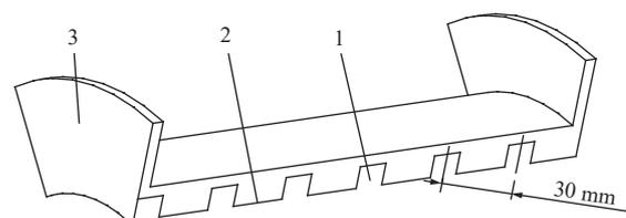
1. Seed pass groove. 2. barrier for removing excessive seeds 3. part for holding the device stationary
