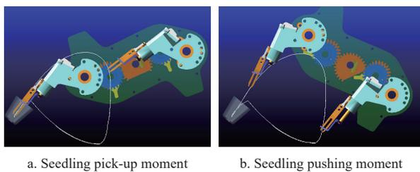
Figure 6 Virtual simulation of the seedling pick-up mechanism
