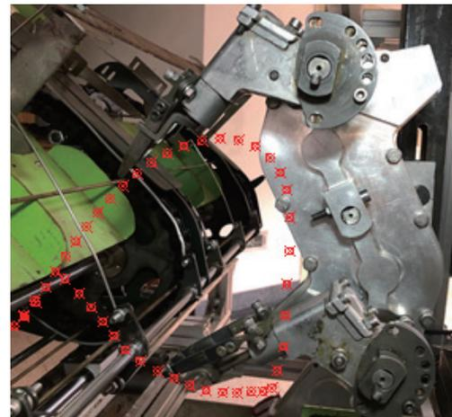
Figure 7 Test trajectory of the seedling pick-up mechanism
