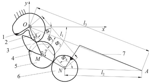
1. First central incomplete non-circular gear 2. Second center incomplete non-circular gear 3. Middle incomplete non-circular gear 4. Middle non-circular gear 5. Third middle non-circular gear 6. Planetary non-circular gear 7. Seedling pick-up arm
