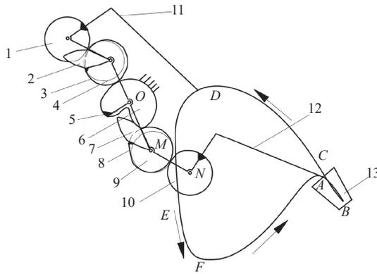
1, 10. Planetary non-circular gears 2, 7. First middle incomplete non-circular gears 3, 8. Second middle non-circular gears 4, 9. Third middle non-circular gears 5. First central incomplete non-circular gear 6. Second central incomplete non-circular gear 11, 13. Seedling pick-up arms 12. Planetary carrier 14. Plug seedling tray
