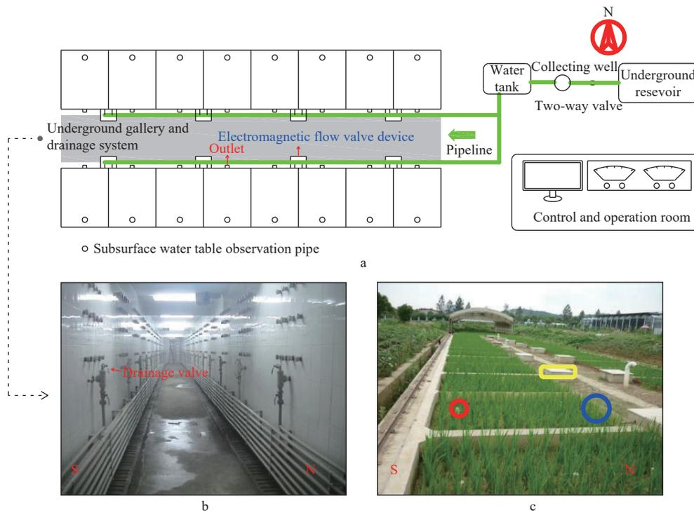
Note: (a) Layout of the study area and experimental management. Water was supplied from an underground reservoir to every fixed tank plot through pipelines. (b) Picture of underground gallery and drainage system. (c) Picture of fixed tank plot. Inside the yellow box is the electromagnetic flow valve device. Inside the red box is the subsurface water table observation pipe. Inside the blue box is the outlet.
