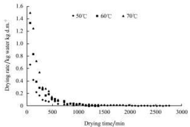
Figure 3 Drying rate changes with moisture ratio of *Syzygium cumini* at 50, 60 and 70 °C
