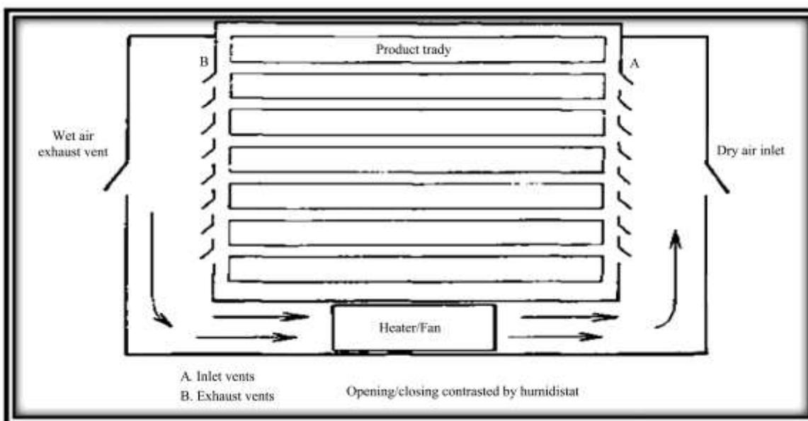
Figure 1 Schematic diagram of tray dryer
