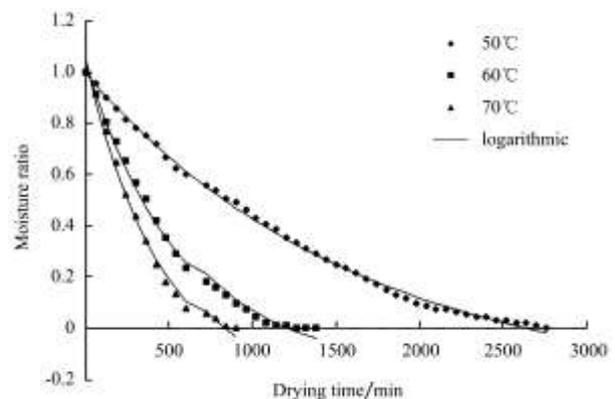
Figure 7 Drying curves of *Syzygium cumini* determined at 50, 60 and 70 °C. Solid curve represents curve fitting using logarithmic model
