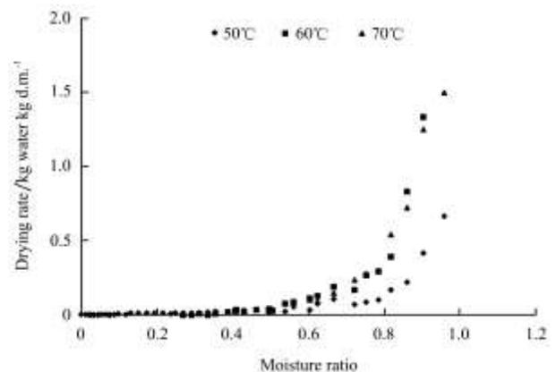
Figure 4 Drying rate changes of *Syzygium cumini* with drying time at 50, 60 and 70 °C
