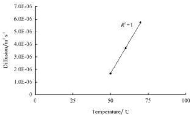
Figure 6 Influence of the drying air temperature on the diffusion coefficient
