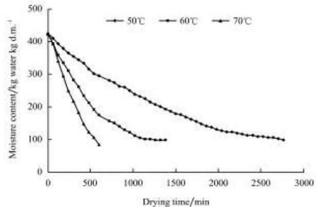
Figure 2 Effects of drying air temperatures at 50, 60 and 70 °C and drying time on the moisture content of *Syzygium cumini*
