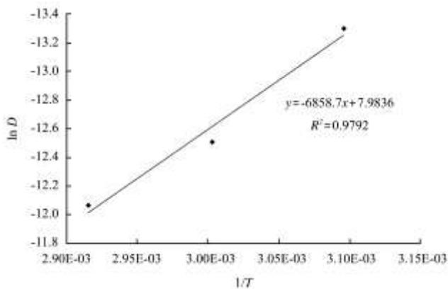
Figure 5 Plot of  $\ln D$  versus  $1/T$  for calculating the activation energy
