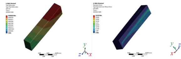
Figure 9 Equivalent cloud chart of turbine output shaft under torsional condition
