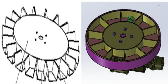
Figure 3 Structural diagram of key components of rotary disc metering device
