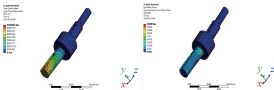
Figure 8 Equivalent cloud chart of flat-head flat key under torsional condition
