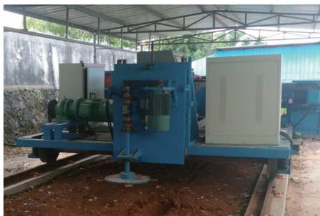
Figure 10 Soil tank test vehicle
