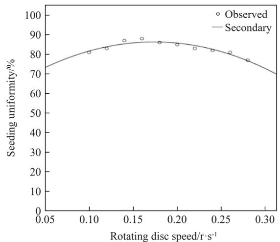
Figure 12 Relation of rotating disc speed and seeding uniformity
