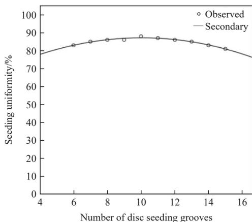
Figure 13 Relation curve of the number of disc seeding grooves and seeding uniformity
