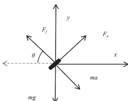
Figure 5 Stress analysis of sugarcane seed in seed guide groove
