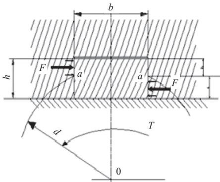
Figure 7 Stress analysis of flat key connection
