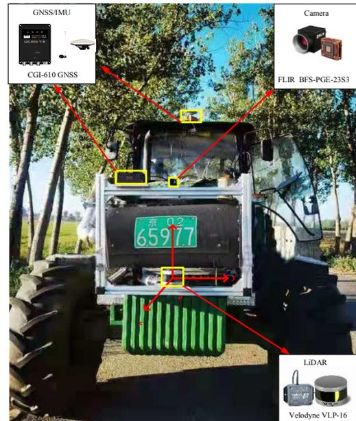
Figure 2 Data acquisition equipment
