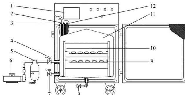
1. Touch screen control panel 2. Material temperature sensor 3. Pressure sensor 4. Vacuum valve 5. Condenser 6. Vacuum pump 7. Air solenoid valve 8. Drain solenoid valve 9. Sample, 10. Far-infrared radiation heating element 11. Drying chamber 12. Infrared-board temperature sensor
