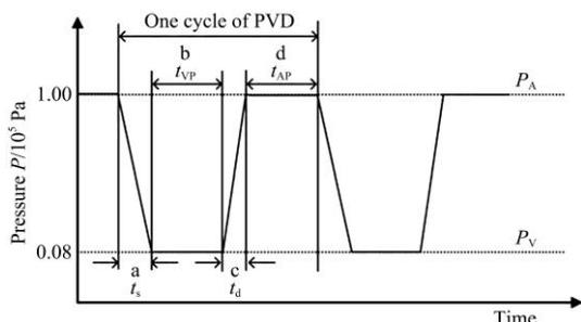
Figure 2 Schematic diagram of drying chamber pressure change kinetics during pulsed vacuum drying
