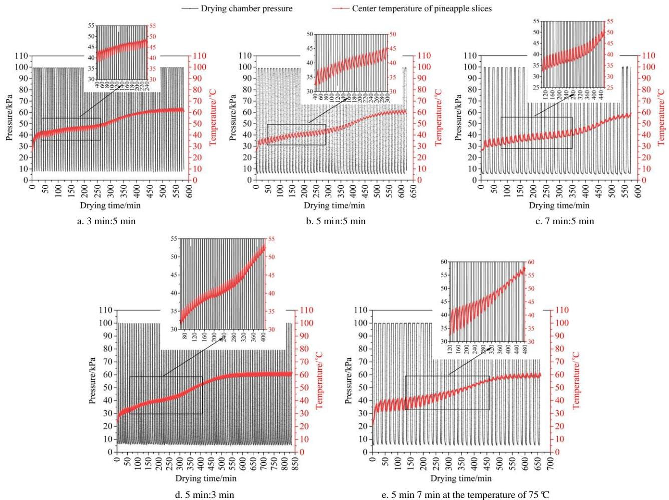
Figure 7 Temperature curves of different pulsed vacuum ratios (PVR)
