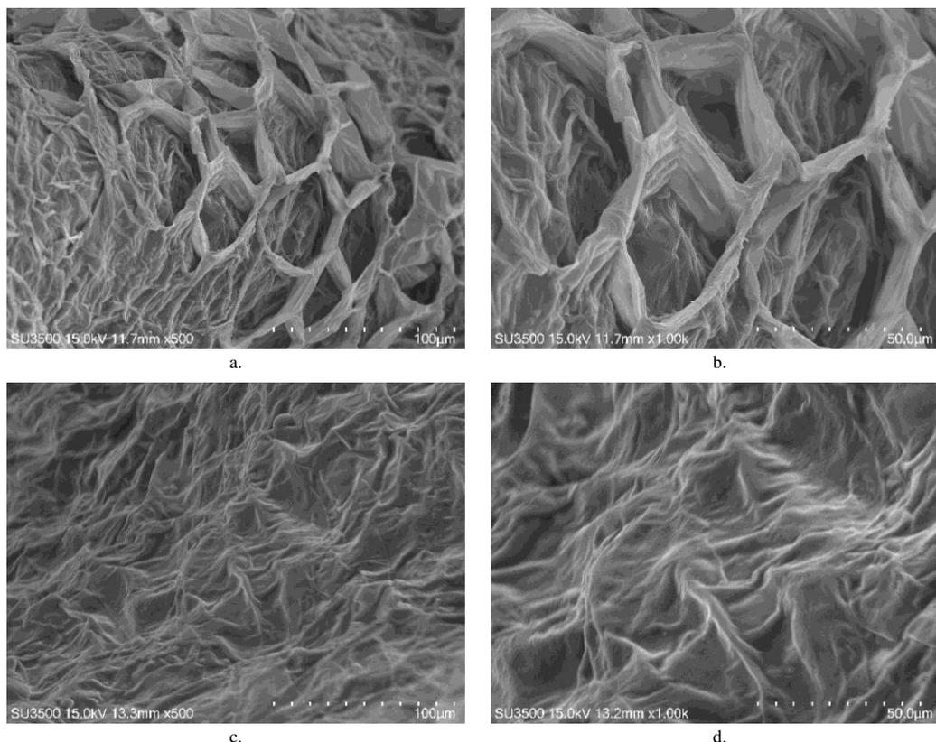
Figure 8 SEM images of pulsed vacuum dried pineapple slices surface in different magnifications (a, b: pulsed vacuum ratio of 5:5 in different magnifications; c, d: pulsed vacuum ratio of 9:5 in different magnifications)
