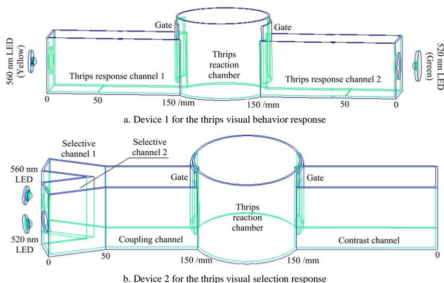
Figure 1 Devices used for investigating the visual response of thrips
