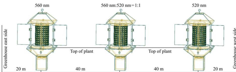
Figure 3 Layout mode of light sources in the greenhouse
