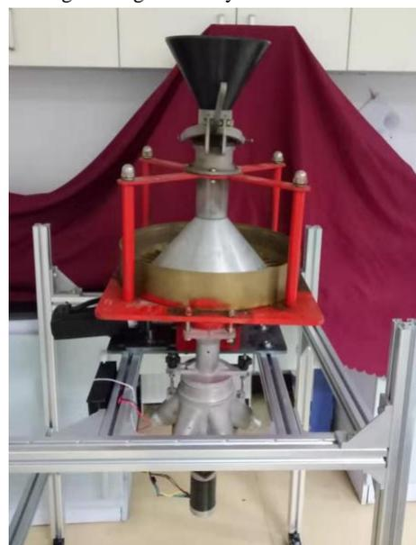
Figure 7 Test bench of plot seeding
