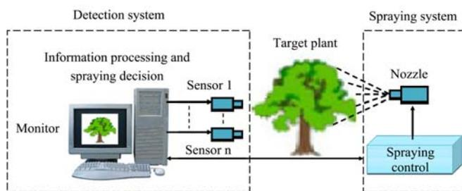
Figure 2 Smart spraying system based on sensing technology
