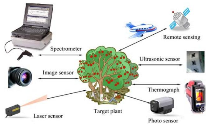
Figure 3 Target detection sensors
