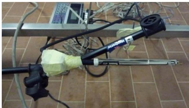
Figure 9 Anemometer (central, 23 cm from floor)
