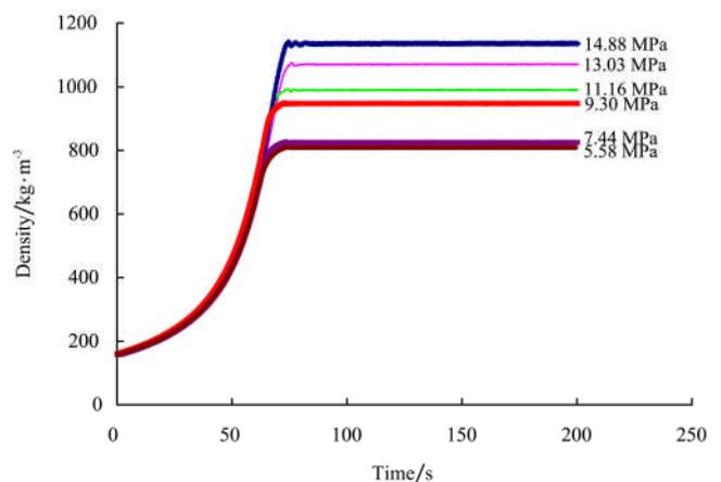
Figure 1 Typical curves of hay density as a function of compression and relaxation time at different preset levels of compression pressures for high quality hay at a moisture content of 10.17% w.b.
