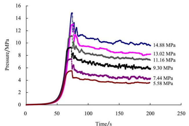
Figure 3 Typical pressure vs. time curves for varying maximum applied pressures during compression and relaxation for high quality timothy hay at 10.17%
