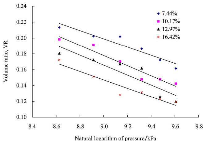
Figure 2 Fitting of Walker's model to the experimental compression data for high quality timothy hay
