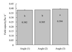
Figure 5 Mean effective field capacity affected by different tilt angles. (means followed by the different letter differ significantly according to Duncan's test)
