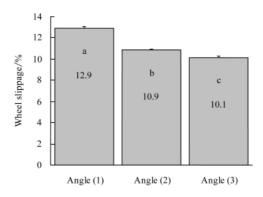
Figure 4 Means wheel slippage affected by different tilt angles.
