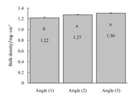
Figure 2 Mean soil bulk density affected by different tilt angles. (means followed by the different letter differ significantly according to Duncan's test)
