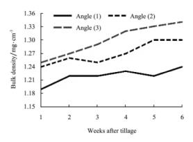
Figure 1 Mean bulk density of surface (0–10 cm) soil, under different tilt angles over time
