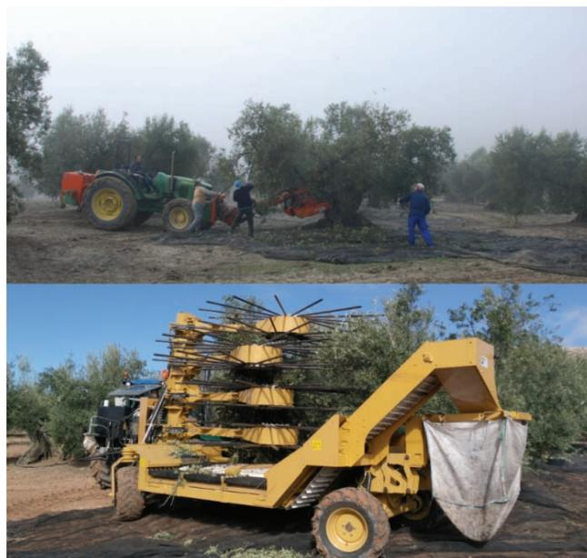
Figure 7 Most common method (trunk shaker and manual canopy beating) used for harvesting (top) and new method (canopy shaker around the tree) (bottom)
