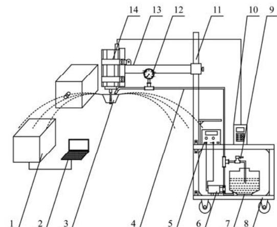
Note: 1. Laser particle size analyzer 2. Laser particle analyzer system 3. Rotary cup atomizer 4. Pipeline 5. DC power 6. Diaphragm pump 7. Tank 8. Support platform 9. Return valve 10. Frequency modulator 11. Lifter 12. Pressure gage 13. Rail 14. Spindle motor
