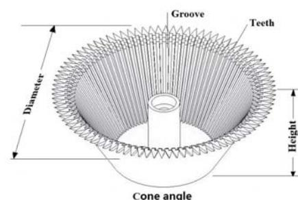
Figure 1 Structural parameters of rotary cup atomizer
