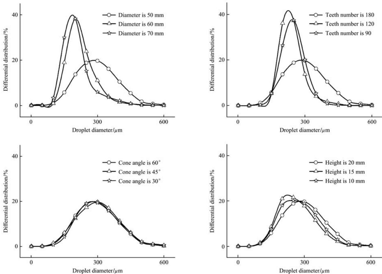
Note:  $D_1$ - $D_3$  are rotary cup with diameters of 50 mm, 60 mm and 70 mm, respectively;  $T_1$ - $T_3$  are rotary cup with teeth numbers of 180, 120 and 90, respectively;  $C_1$ - $C_3$  are rotary cup with cone angles of 60°, 45° and 30°, respectively;  $H_1$ - $H_3$  are rotary cup with heights of 20 mm, 15 mm and 10 mm, respectively, the same below.
