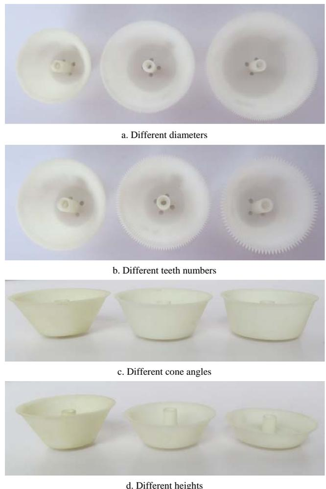
Figure 3 Rotary cups with different structure parameters
