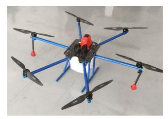
Figure 1 SLK-5 plant protection UAV
