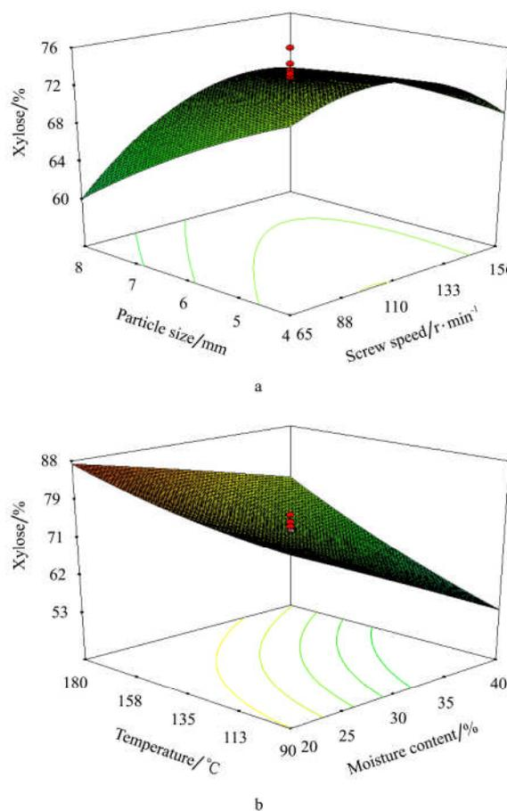
Figure 2 Effect of independent variables interaction on xylose recovery (when other factors fixed at the center point)
