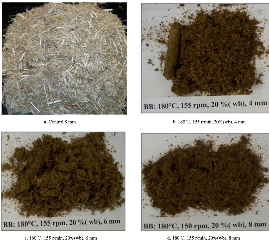
Figure 5 Big bluestem pretreated at optimum and validated conditions
