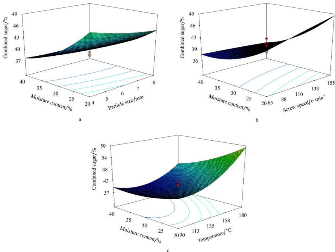
Figure 3 Effect of independent variables interaction on combined sugar recovery (when other factors fixed at the center point)
