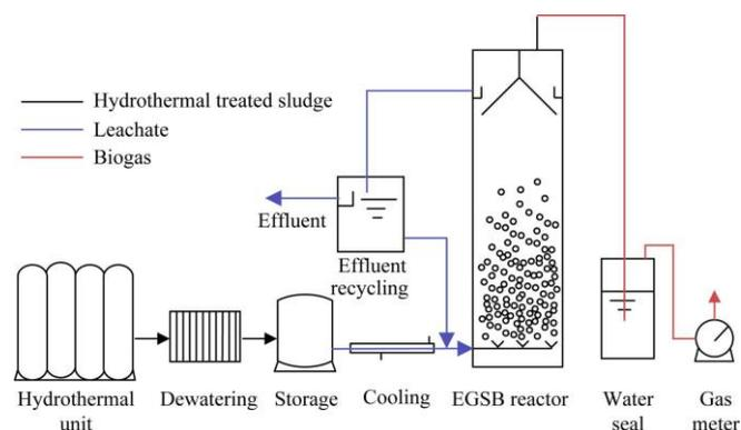
Figure 1 Scheme of pilot EGSB process
