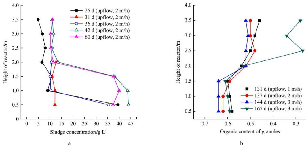
Figure 5 Distribution of sludge in EGSB reactor
