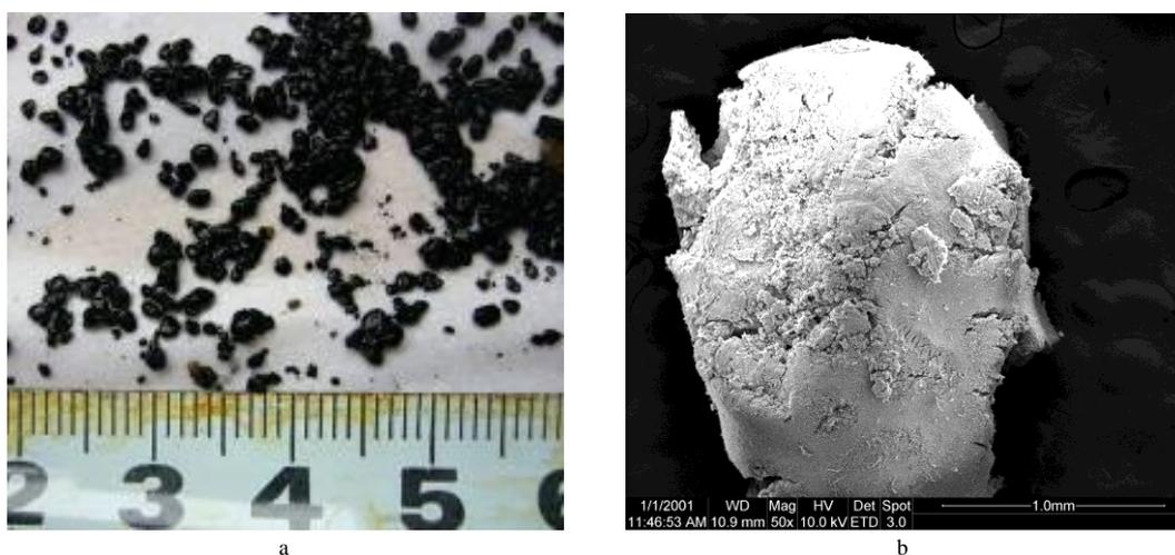
Figure 6 Picture of granular sludge (a) photo of granules at 98 day; (b) SEM photo of granules at 98 day
