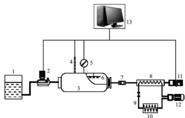
Note: 1. Water tank 2. Water pump 3. Vacuum chamber 4. Thermometer 5. Piezometer 6. Water sprayer 7. Check valve 8. Steam condenser 9. Throttle valve 10. Condenser 11. Vacuum pump 12. Compressor 13. Computer
