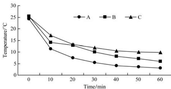
Figure 2 The temperature profiles of broccoli as a function of treatment time according to the vacuum cooling (A), cooling water (B), and cold room (C) treatments
