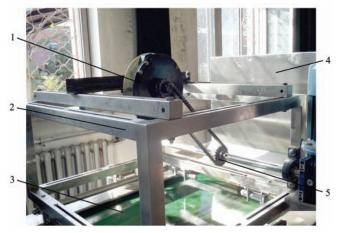
1. Pickup finger precision maize seed metering device 2. Test bench 3. Seed bed 4. Image acquisition processing equipment 5. Transmission system Figure 11 Actual operation of verification experiment
