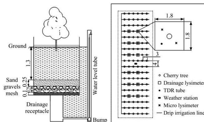
Figure 1 Experimental arrangement and schematic diagram of lysimeter (m)
