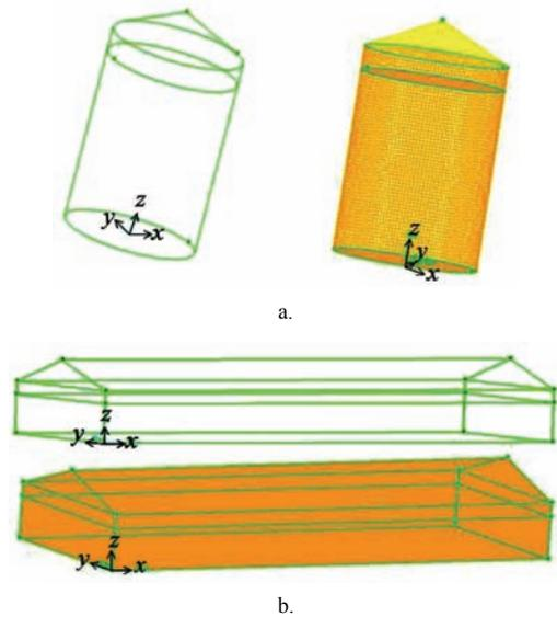
Figure 2 Geometric system studied and the 3-D computational domain of (a) squat silo and (b) large size horizontal warehouse
