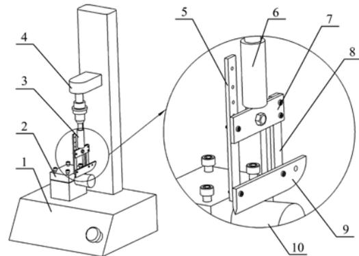
1. Universal testing machine 2. Clamp 3. Knife carriage 4. Sensors
