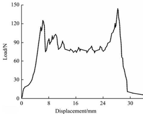
Figure 2 Typically experimental curve of the vertical cutting force
