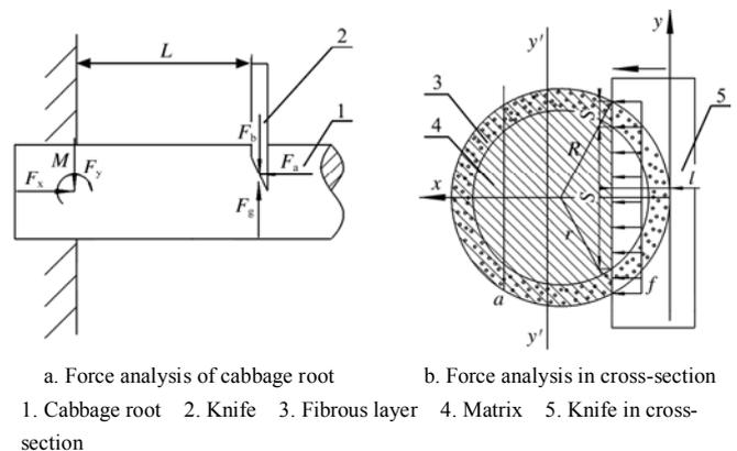
Note: a-a is the working axis; y'-y' is the neutral axis; x is the x coordinate; y is the y coordinate.
