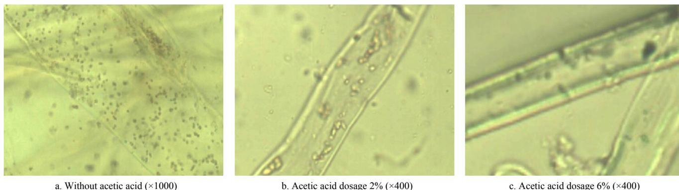
Figure 2 Surface morphology of crude cellulose fiber with different acetic acid dosages
