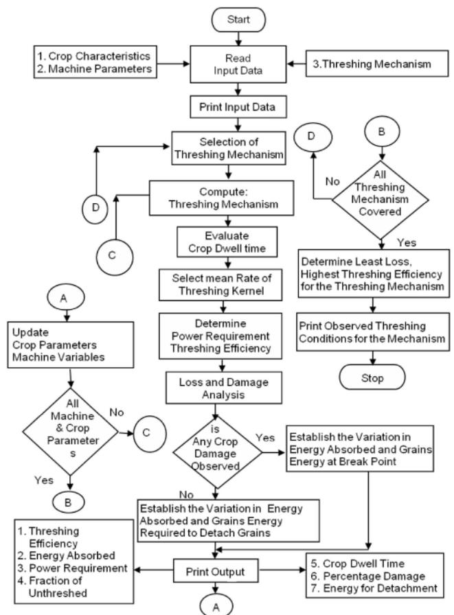
Figure 4 Flow chart for the programme for the simulation of threshing process
