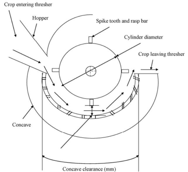
Figure 1 Cylinder concave arrangement of a combined spike tooth and rasp bar thresher mechanism
