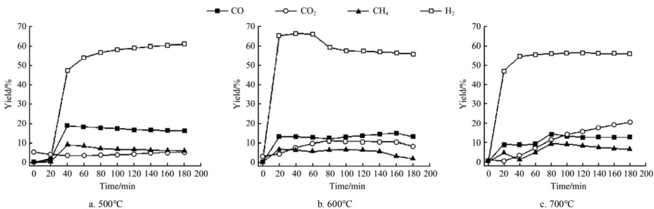
Figure 6 SR of bio-oil at various temperatures with 30.5% Ni/ $\gamma$ -Al<sub>2</sub>O<sub>3</sub> catalysts
