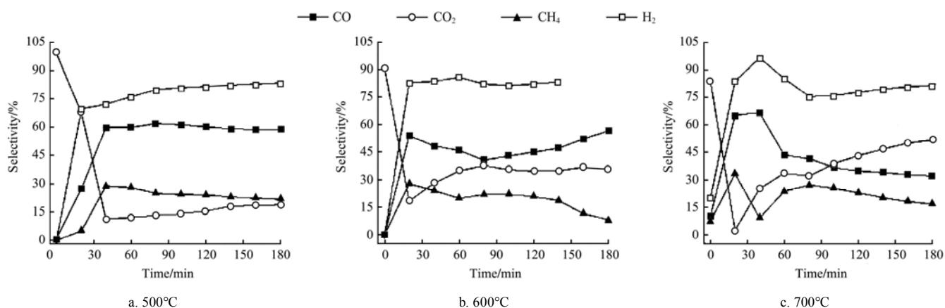
Figure 7 Effect of temperature on gaseous selectivity of steam reforming SR of bio-oil
