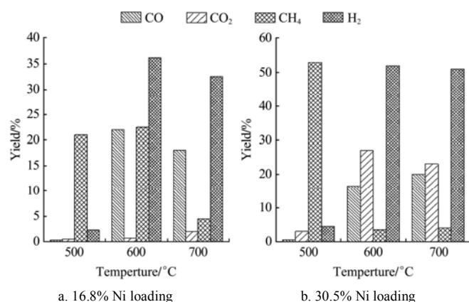
Figure 2 Yields of gas products from SR of acetic acid over catalysts with different Ni loadings
