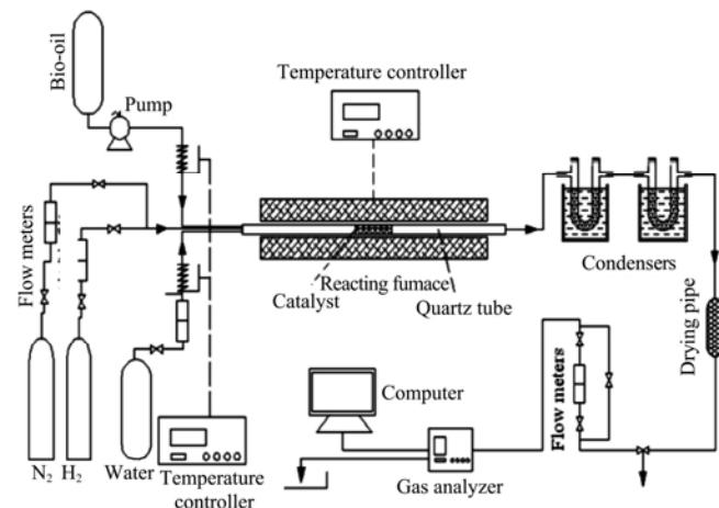
Figure 1 Schematic diagram of laboratory-scale apparatus used for catalytic steam reforming
