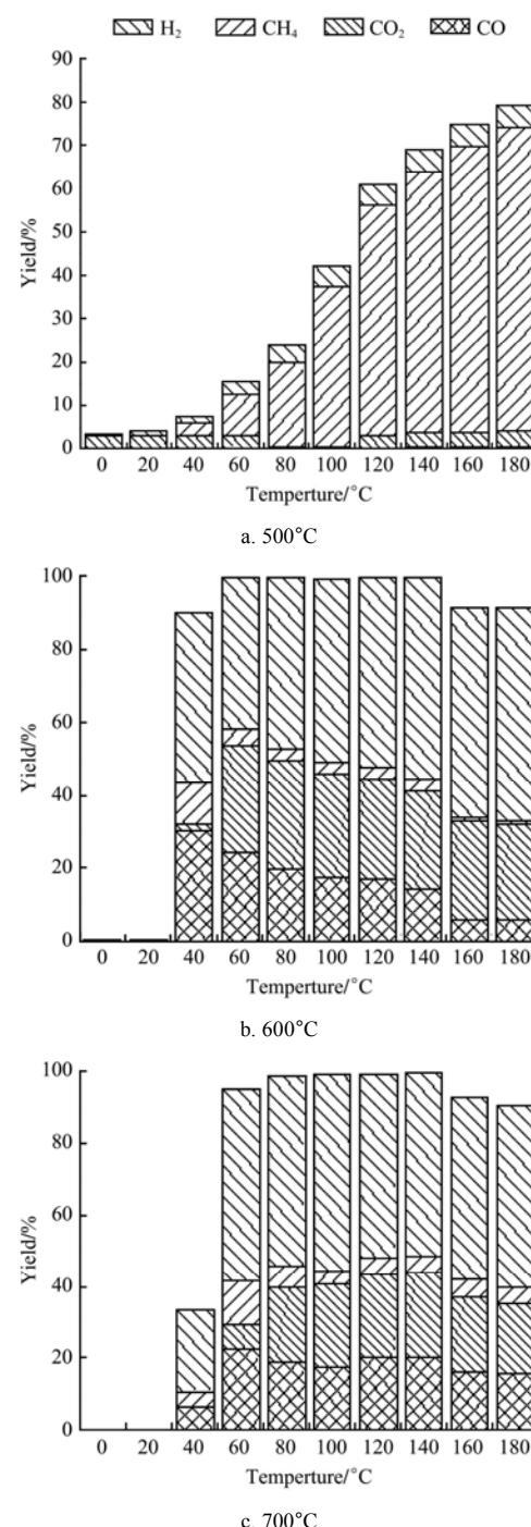
Figure 4 Yields of gas products from SR of acetic acid at different temperatures with catalyst of 30.5% Ni/γ-Al<sub>2</sub>O<sub>3</sub>
