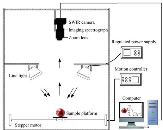
Figure 1 Schematic of the shortwave infrared hyperspectral imaging system for apple fruit
