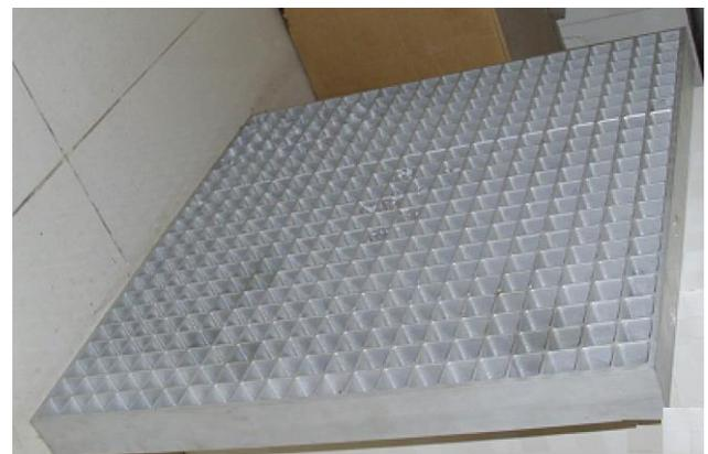
Figure 5 Square two-dimensional nozzle flow measurement device
