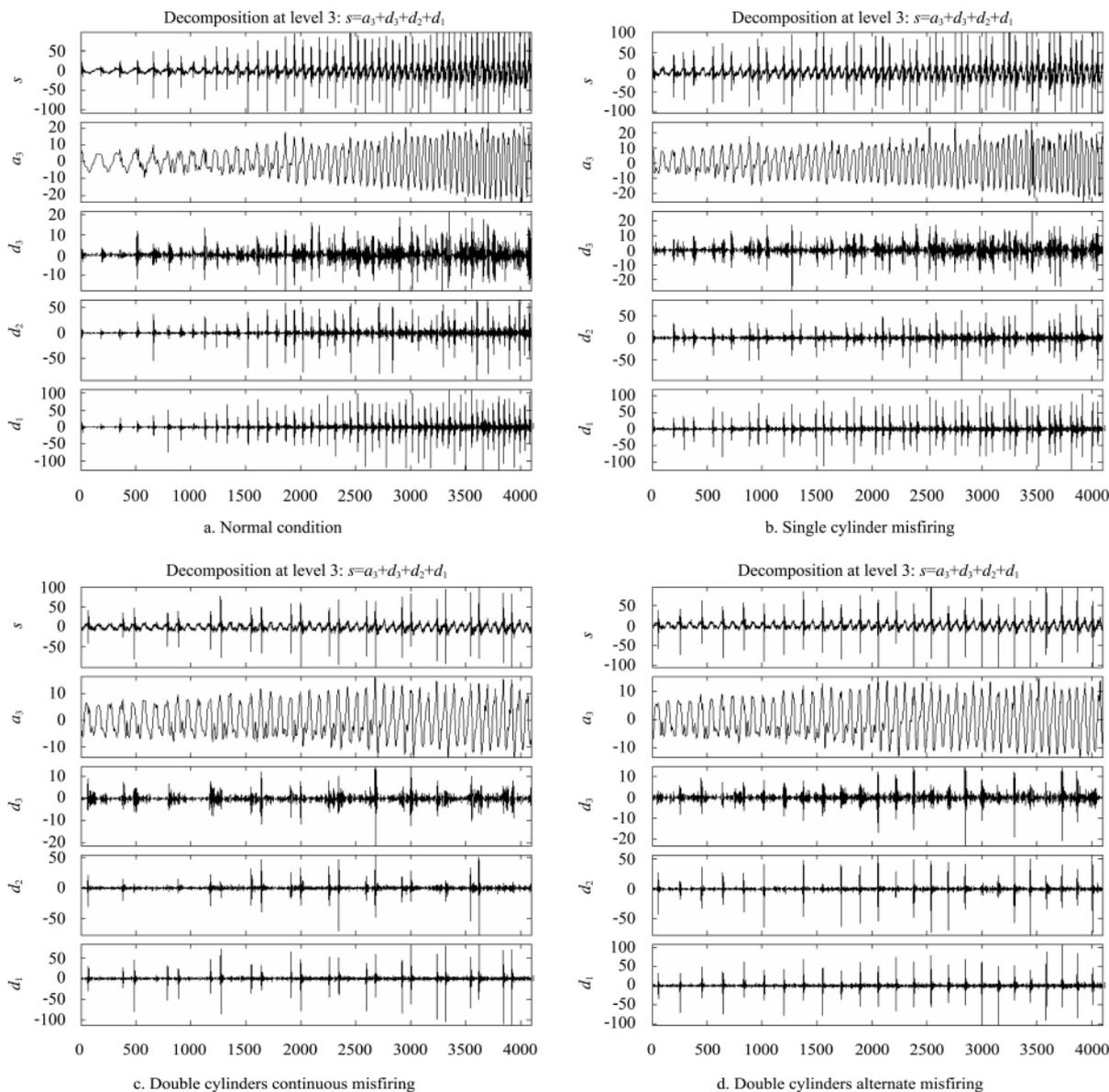
Fig.4 Wavelet decomposition of vibration signals under four conditions in accelerate section
