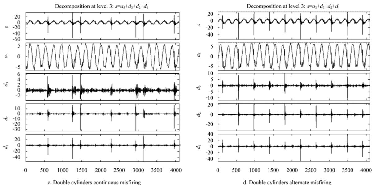
Fig.3 Wavelet decomposition of vibration signals under four conditions in idle section
