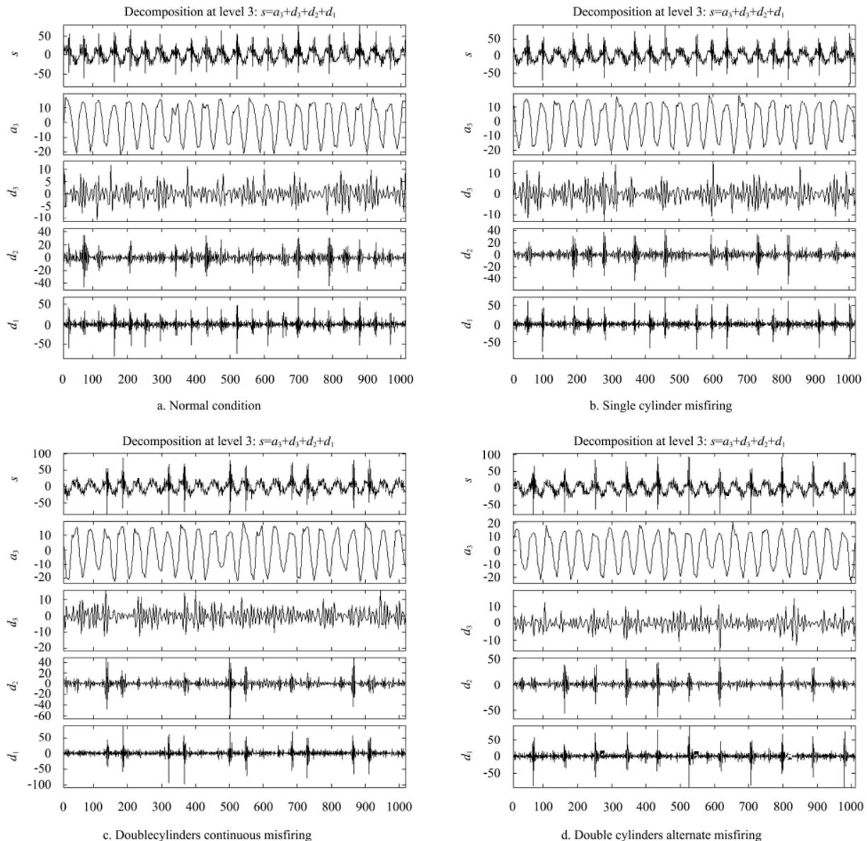
Fig.5 Wavelet decomposition of vibration signals under four conditions in high speed section
