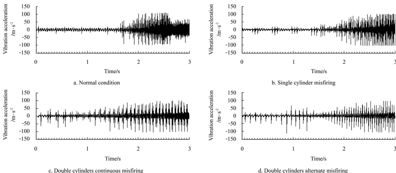
Fig.2 Vibration acceleration signals of four conditions
