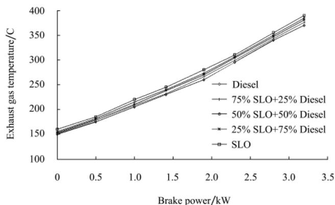
Figure 4 Variation of exhaust gas temperature with brake power for different diesel-sea lemon oil blends
