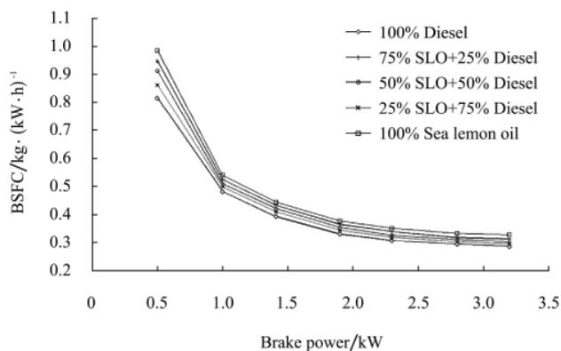
Figure 2 Variation of BSFC with brake power for different diesel-sea lemon oil blends
