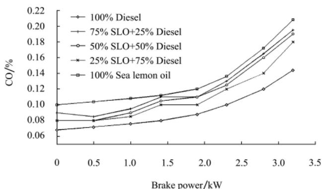
Figure 6 Variation of CO with brake power for different diesel-sea lemon oil blends
