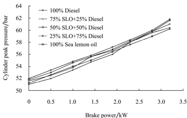
Figure 9 Variation of cylinder peak pressure with brake power for different diesel-sea lemon oil blends
