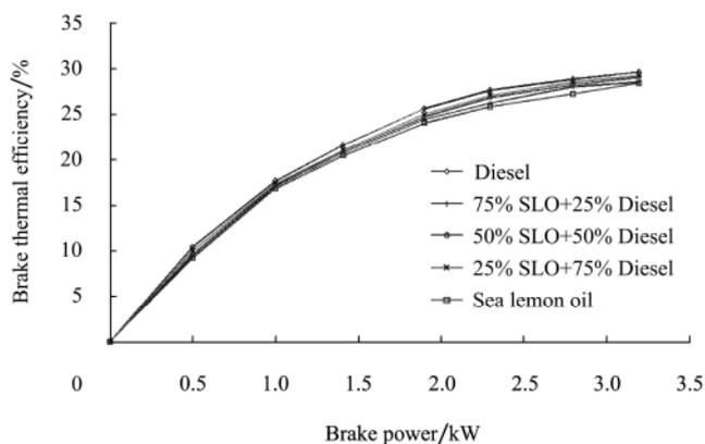
Figure 3 Variation of brake thermal efficiency with brake power for various diesel-sea lemon oil blends at optimum injection timings
