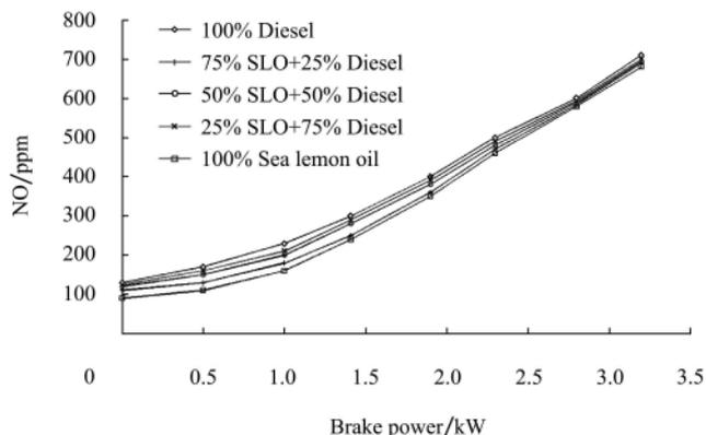
Figure 7 Variation of NO with brake power for different diesel-sea lemon oil blends
