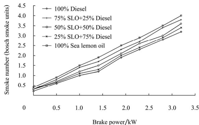
Figure 8 Variation of smoke number with brake power for different diesel-sea lemon oil blends
