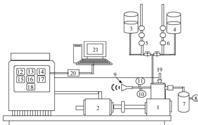
1.Engine 2.Dynamometer 3.Sea Lemon Oil Tank 4.Diesel Tank 5.Burette (Sea Lemon Oil) 6.Burette (Diesel) 7. Air Tank 8. Air Filter 9.Silencer 10.Smoke Pump 11.Exhaust Gas Analyzer 12.Fuel Flow Rate Indicator 13.RPM Indicator 14.Air Flow Rate Indicator 15.Exhaust gas Temp. Indicator 16.Coolant Temp. Indicator 17.Lube oil Temp. Indicator 18.Water Flow Rate Indicator 19.Pressure Sensor 20.Charge Amplifier 21.Digital Data Acquisition System
