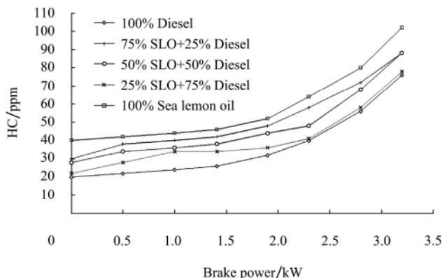
Figure 5 Variation of HC with brake power for different diesel-sea lemon oil blends
